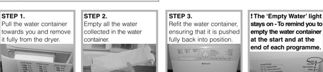
I Failure to empty the water container will result in:
